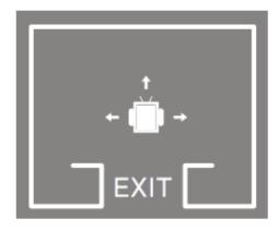
This challenge features a four sided, enclosed box with one opening large enough for your robot to exit. The challenge is to have the robot escape the box in as little time as possible using any features available to you. A light source will be located outside the exit. The starting point for all robots will be the center of the box, with the robot pointed in one of three random directions.
